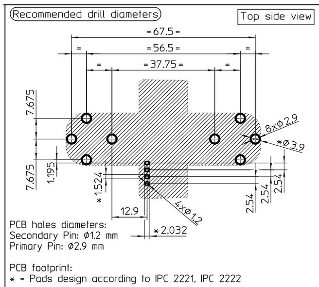
Dimensions (in mm, general tolerance  $\pm 0.3$  mm)
